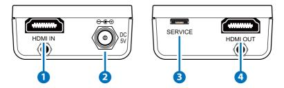
**1 HDMI IN:** Connect to HDMI source equipment such as a media player, game console or set-top box. DVI sources are supported with the use of an HDMI to DVI adapter.
