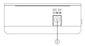
① DC 5V: This slot is where you plug the 5V DC power supply into the unit and connect the adaptor to an AC wall outlet.
