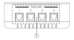
① Optical In: These slots are to connect with input source equipments such as DVD/Blue-Ray player for audio input signal sending.
