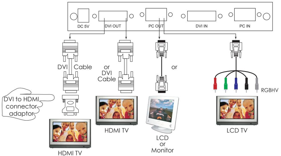
The HTCP-255D can output a variety of PC, SD and HD resolutions in both digital analog format simultaneously.
