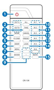
**Select to VIEW ALL:** Press from INPUT 1~6 or MUTE to select input sources for main channel.
