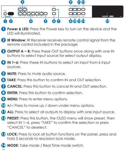
**(LCM:** Display input and output selection and menu options.
