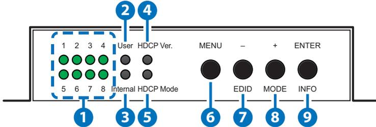
**1 LEDs 1~8:** These LEDs illuminate to indicate which EDID from the currently selected EDID mode is active.
