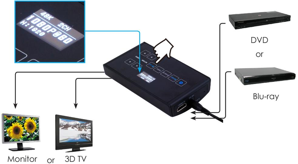
For checking display's support timing, connect HDMI output only to the display and press the PATTERN and TIMING button.
