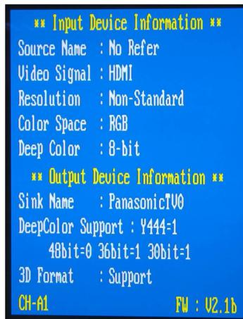
Press [M/↵] to check the input/output device information and software version.
