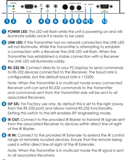
**7 IR WINDOW:** Accepts IR signals from any standard remote control and sends the signal to the IR Out on the associated Receiver.
