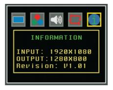
Displaying both input source and output display timing with software version.
