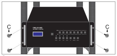
4 Use four Flanged screws to attach the 8x8 Matrix to the rack frame.
