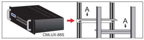
3 Slide the device on top of the L-Shaped rails.
