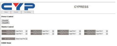
Click on the 'User Setting' tab allows you to reset the IP configuration. The system will ask for a reboot of the device every time any of the settings are changed. The IP address needed to access the Web GUI control will also need to be changed accordingly on the web address entry bar.
