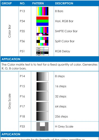
This is used to locate faulty linearity of the video amplifier or greyscale setting. Nonlinearities mainly result in a compression of the white level.
