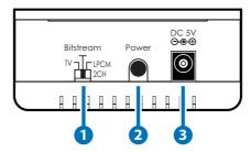
1 Audio EDID Switch: This switch allows users to select which audio EDID settings are used for audio output.
