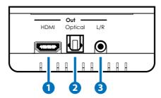
1 HDMI Out: Connect the HDMI output port to the HDMI input port of your display with an HDMI cable.
