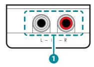
1 L/R IN: Connect this input to the stereo output of an audio streamer, AV receiver, LCD TV, or DVD player, using stereo RCA cables.
