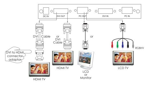
The HTCP-255D can output a variety of PC, SD and HD resolutions in both digital analog format simultaneously.
