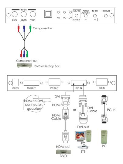
The HTCP-255D accepts component, PC and DVI inputs. The formats supported by these inputs are as follows:
