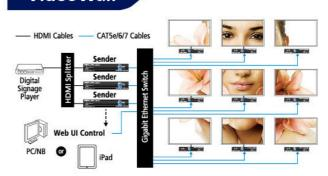
\* Video Wall function need PB5000-S+ Sender & PB5000-R+ to co-work.
