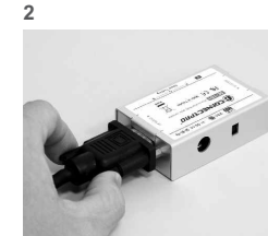
2 Connect VGA cable from display to black VGA port
