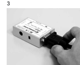
3 Connect VGA cable between system and blue VGA port
