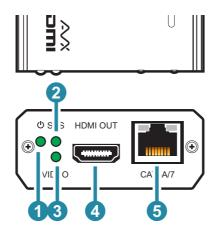
1 Power (也) LED: This LED will illuminate to indicate the unit is on and receiving power.
