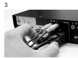
Connect displays video ports 1. Video cables 2. Audio cables
